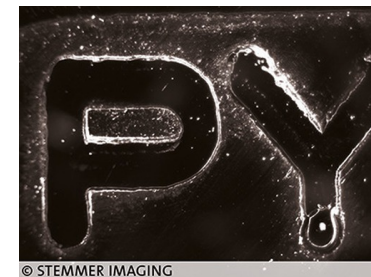
lens with small depth of field removes scratches
