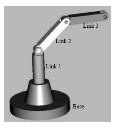
Mechanics of a manipulator can be represented as a kinematic chain of rigid bodies (links) connected by revolute or prismatic joints.
