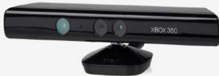
Kinect v1 : based on triangulation
