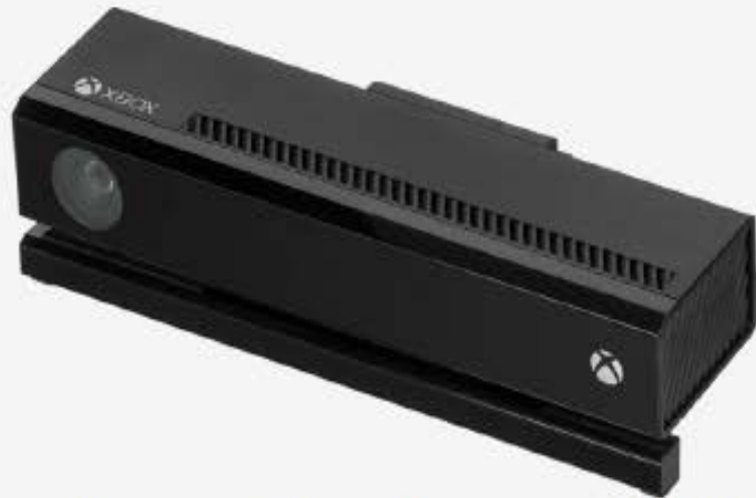
Kinect v2 : based on time of flight
