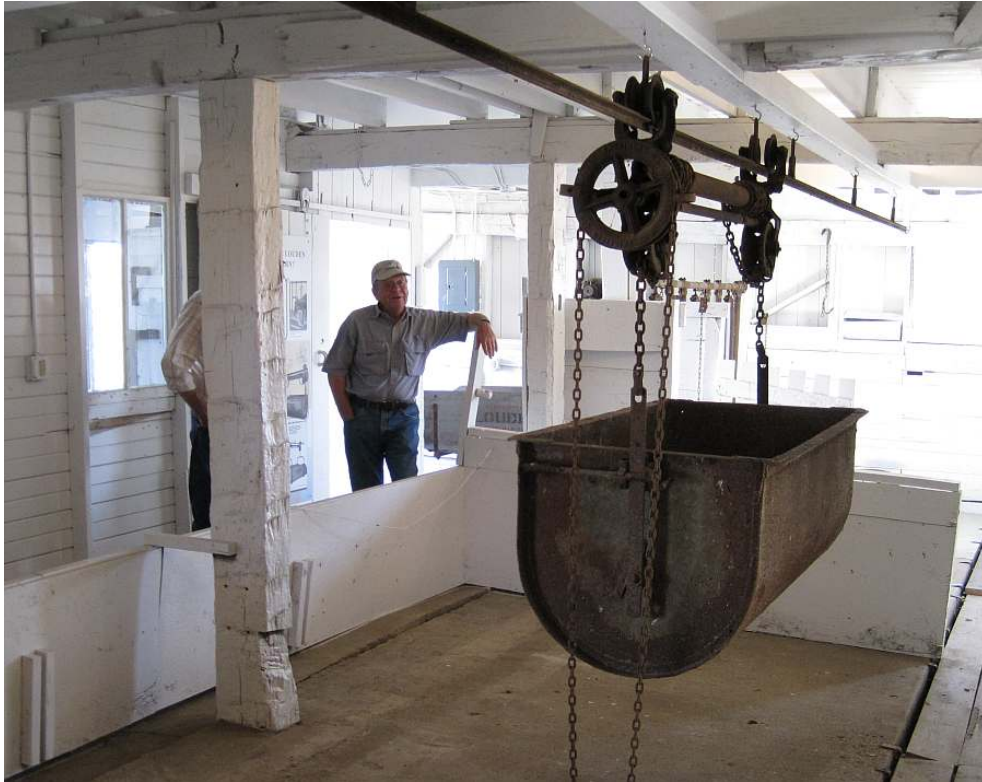
Cow stable mechanization – manure carrier.
