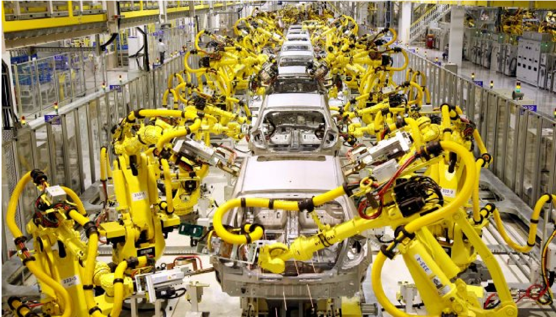
Automotive plant KIA Žilina, Hyundai industrial robots.
