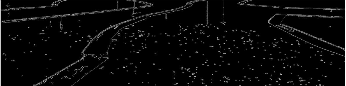
Figure 2.3: Canny edge detection example
